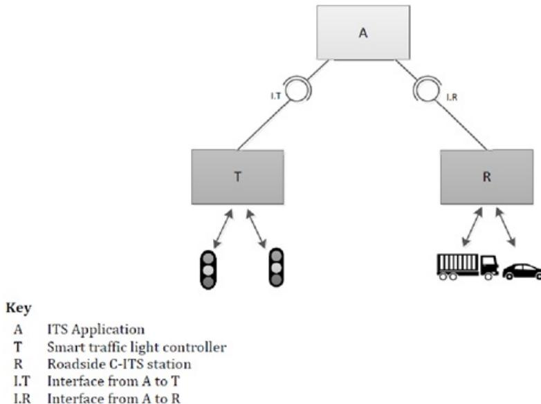
**Figure 1 — iTLC: architecture for connected roadside units (example)**
